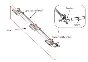
Turn the clamp screws to fix the jig-support to the door, place the first jig into the jig-support casing.
