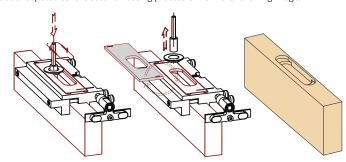
Remove the clamp support, rotate and insert it into the cases, like in the following diagram: 1 2 3
